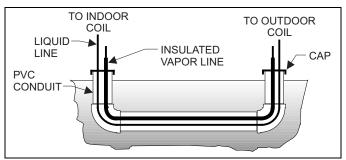
FIGURE 3: Underground Installation
